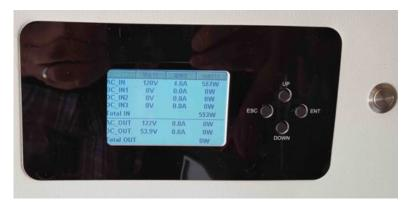
Verify the OGS's LED shows DC IN (if connected to DC power {Solar/PV, other}) by pushing the DOWN button (R-hand side of the LCD display).
