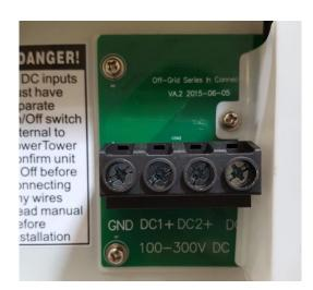
Connect the hot wire from the solar panels/combiner boxes to the "DC1+ or DC2+ or DC3+" terminal. Tighten the screw terminal to 16 inch-pounds.
