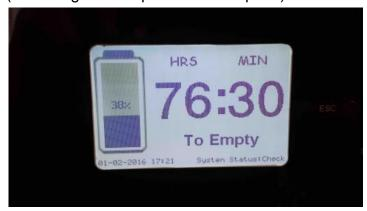
The example above shows battery capacity of 38% and 76hrs 30min.
