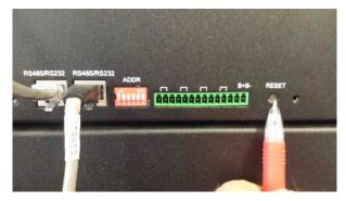
Remove pencil/pen. The top battery LED indicator lights will begin to blink. As communication is established the other batteries will begin to be activated and their respective LED lights will begin to blink.
