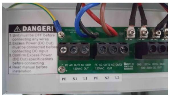
Route the cable and conduit from the AC (LOAD SIDE) distribution panel to the OGS's AC (OUTPUT) conduit.
